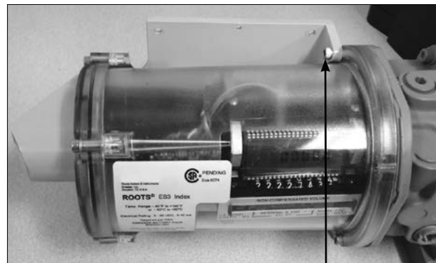
Figure 12 - Insert the 7/8" (long) screws 7/8" screws (one not shown)
