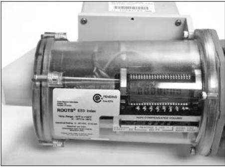
Figure 29 - Top inlet: notice the space between the ES3 label and the bracket
