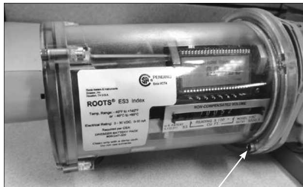
Figure 9 - Leave screw under odometer in place
