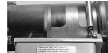
Figure 26- Attach AMR to ES3 bracket
