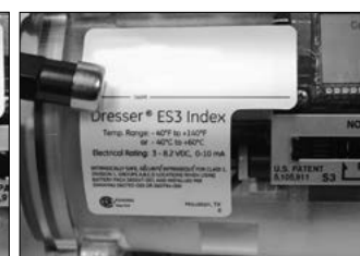
Figure 2 - Swipe magnet across the "swipe line" to change the screen displays
