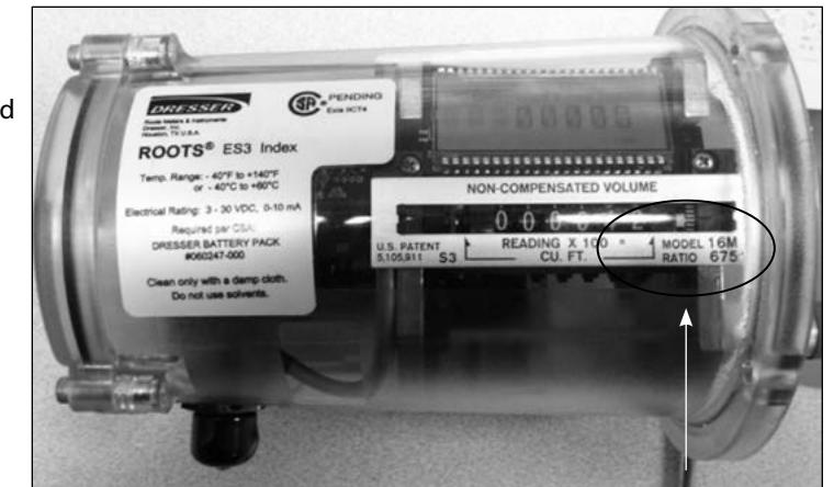
Figure 12.1 - Location of meter size and gear ratio Meter size = 16M Ratio = 675
