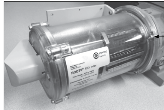
Figure 10.26 - Insert remaining 3/4 inch (short) screws
