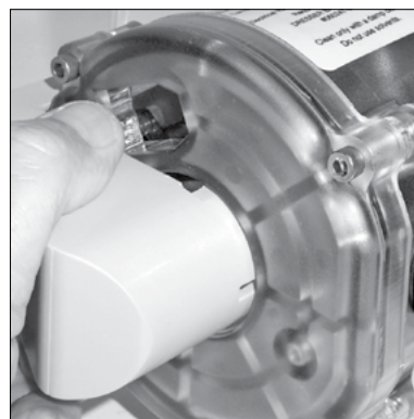
Figure 10.24 - Place cable gland connector into recess
