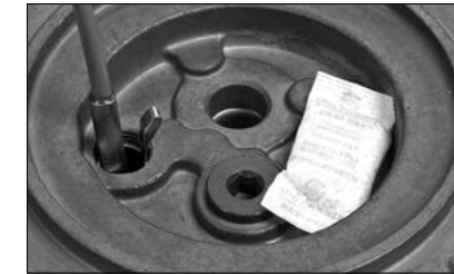
Figure 10.10 - Insert Temperature probe
