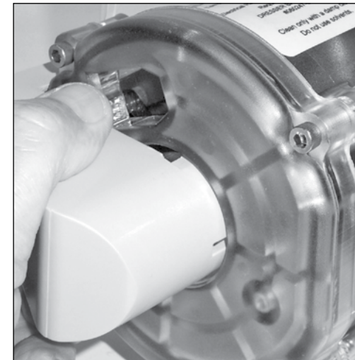
Figure 10.28 - Place cable gland connector into recess
