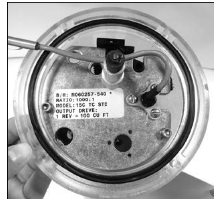
Figure 10.19 - Quad-Ring seal in circular groove
