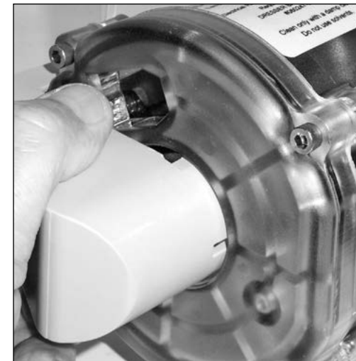
Figure 10.38 - Place cable gland connector into recess
