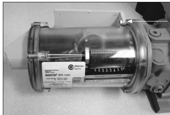
Figure 10.36 - Insert the 7/8-inch (long) screws
