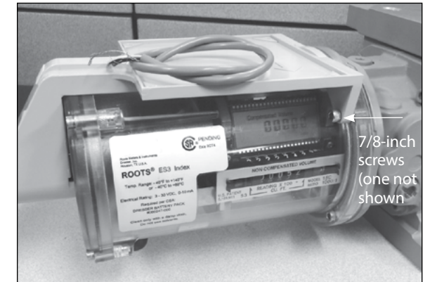
Figure 10.29 - Insert the 7/8-inch (long) screws
