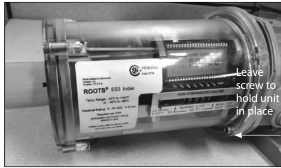
Figure 10.34 - Leave screw under odometer in place
