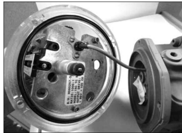
Figure 13.9 - Remove grommet securing previous probe; remove plate for probe
