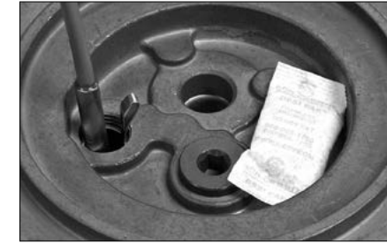
Figure 10.20 - Insert Temperature probe
