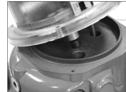
Figure 10.11 - Seat magnet in magnet well
