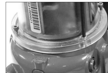
Figure 10.12 - Torque mounting screws to a maximum of 12-14 inch-pounds
