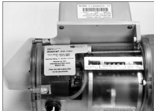
Figure 11.16 - Side inlet: notice the close positioning of the ES3 label to the bracket
