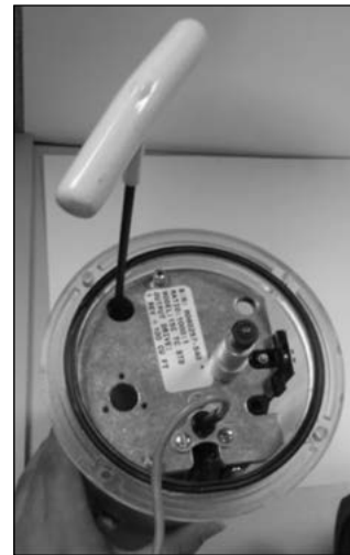
Figure 13.10 - Remove single screw holding counter to unit
