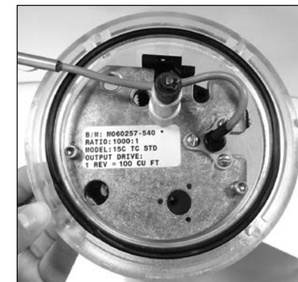
Figure 10.9 - Quad-Ring seal in circular groove
