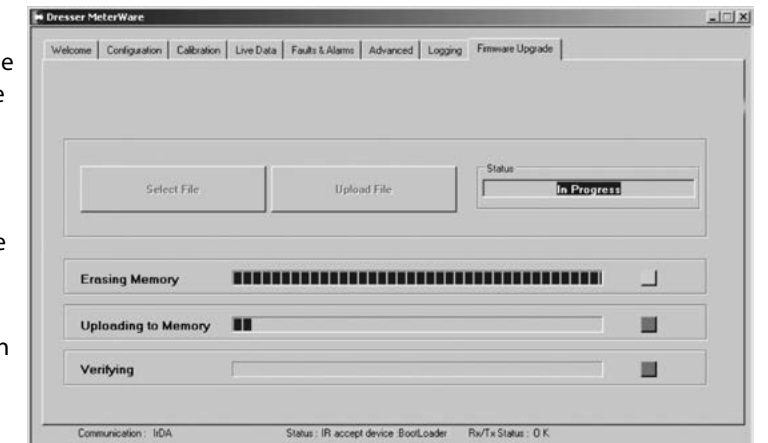
Figure 15.8 - Progression of three steps for uploading the new firmware to the unit
