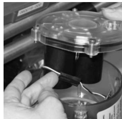
Figure 13.3 -Remove excess slack: circular version
