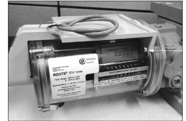
Figure 10.39 - Insert the 7/8-inch (long) screws
