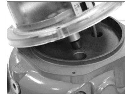
Figure 10.21 - Seat magnet in magnet well
