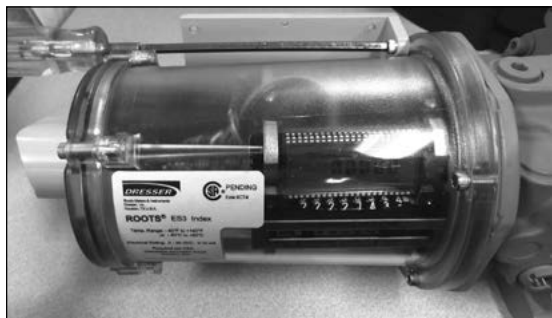
Figure 10.32 -Remove screws attached to AMR bracket
