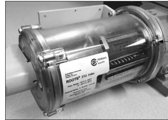
Figure 10.37 - Insert the 3/4-inch (short) screw
