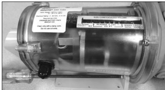
Figure 10.33 - Remove screws attached to AMR bracket
