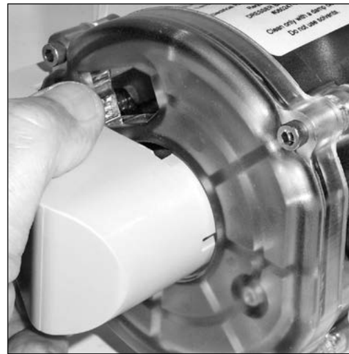
Figure 10.35 - Place cable gland connector into recess
