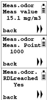
A memory entry consists of the saved entries for measured value, measuring point number and warning odour. The date and time of the measurement have already been displayed in the memory directory. It is not possible to subsequently amend any memory entries. The 'Menu (on/off)' key returns you to the memory management.
