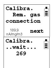
The measuring cap can now be removed and the calibration gas bottle is closed. F2 (continue) takes you to the sensor regeneration.
